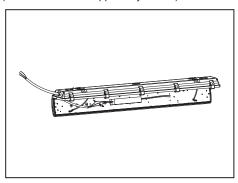
2. Secure mounting clips to housing recesses by firmly pressing them into place until both sides of the clip are secured.
