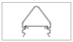
Secure mounting clips to housing recesses by firmly pressing them into place until both sides of the clip are secured. Hang fixture from customer supplied chain using V-brackets.
