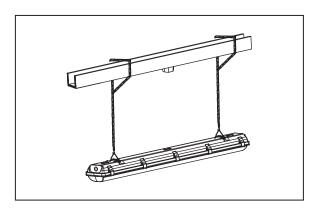
4. Release latches by pulling top of latch away from housing
