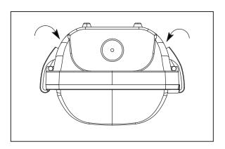
Connect power to driver as shown in the figure. (The flexible cord supplied by others)
