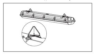
3. Hang fixture from customer supplied chain using V-brackets.
