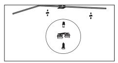
3. Release latches by pulling top of latch away from housing.
