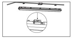
4. Without touching LED boards,detach LED tray and lens from fixture.
