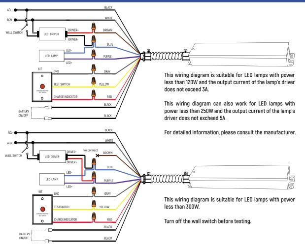
The emergency LED driver contains a control/monitor circuit which will perform a 40-second discharge test once a month, and a fully discharge te test once a year. At this time, the unit will simulate an AC power faulure and automatically switch to emergency mode. During routine testing, the unit will monitor the operation of the LED load, battery voltage, and emergency duration, and if the unit detects any problems, the indicator will flash quickly.
