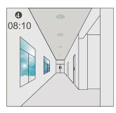
When the ambient light exceeds set point off to light, the light will turn OFF even if when the space is occupied.
