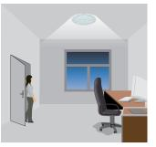
With insufficient ambient light, the sensor switches ON the light automatically with the presence of motion.
