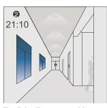
The light dims to stand-by level after the hold-time.
