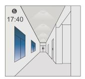
The light automatically turns ON at 10% when ambient light is insufficient (no motion).
