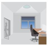
After hold time has elapsed, the light dims to stand-by level if the surrounding ambient light is below the daylight threshold.
