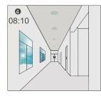
When the natural light exceeds set point off to light, the light will turn OFF even if when the space is occupied.
