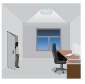
With insufficient ambient light, the sensor switches ON the light automatically when motion is detected.
