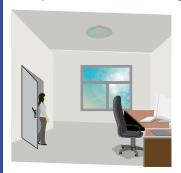
With sufficient ambient light, the light does not switch ON when motion is detected.
