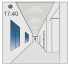
The light automatically turns 0N at 10% when natural light is insufficient (no motion).
