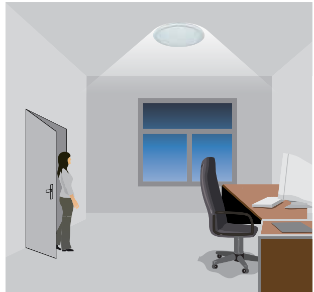
With insufficient ambient light, the sensor switches the light ON automatically when a person enters the room.
