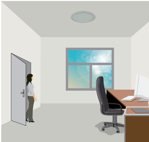
With sufficient ambient light, the light does not switch ON when presence is detected.
